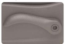
To adjust the driver or front passenger seatbacks, lift the lever on the outboard side of the seat cushion. Release the lever to lock the seatback. To position the seatback in a vertical position, lift the lever without pushing on the seatback.
